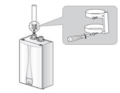
Notice Tighten the screws and fix the vent clip.
