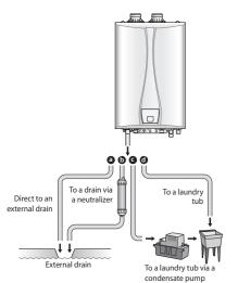
(a) From the water heater directly into an external drain.
