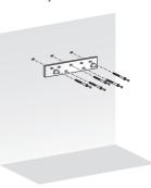
3 Align the grooves on the back of the boiler with the tongues on the mounting bracket and hang the boiler from the bracket.
