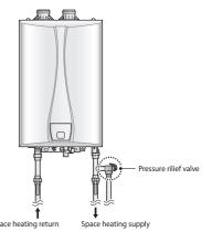
If the pressure relief valve discharges hot water periodically, thermal expansion may occur due to an expansion tank problem or small expansion tank size. Do not plug the pressure relief valve
